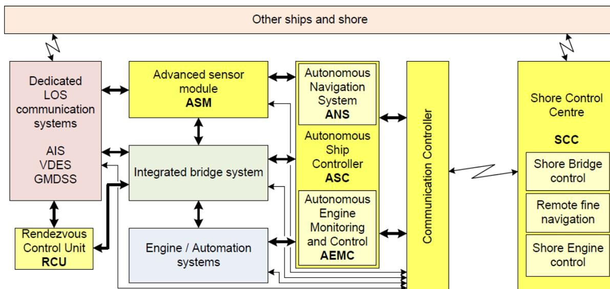
**Figure 1: Overview of the high level modules /2/**
