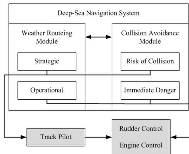
**Figure 4: Autonomous navigation system architecture /7/**
